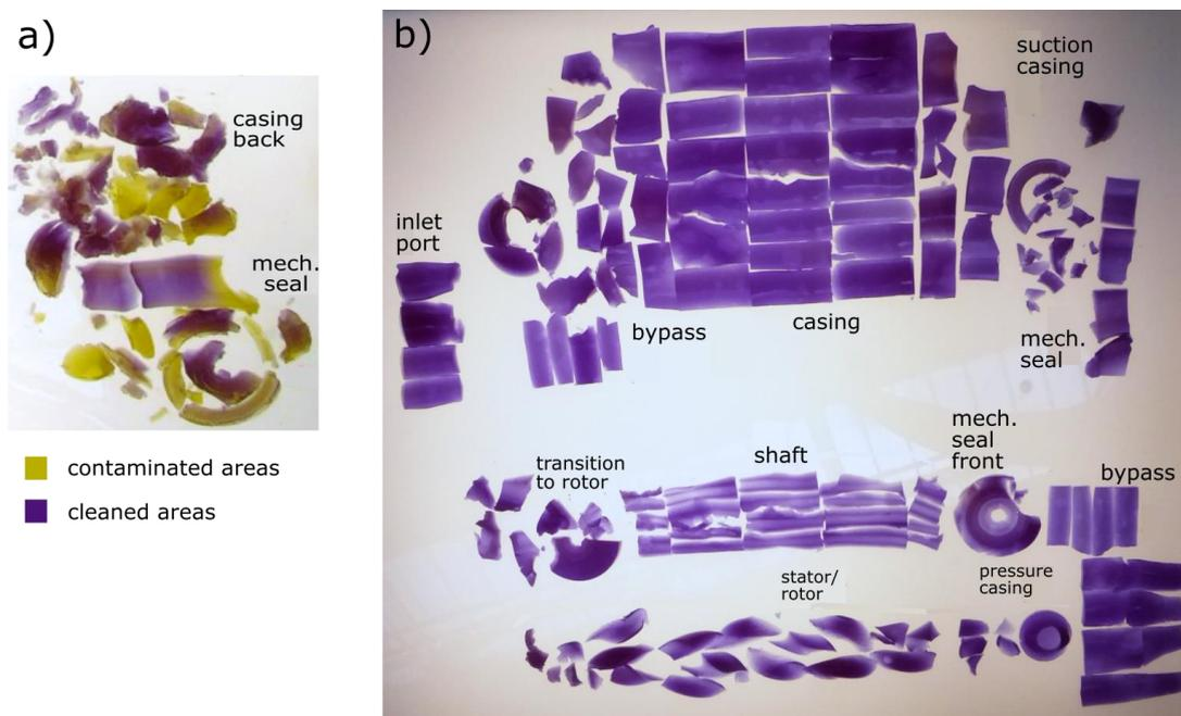
Fig.3: EHEDG cleaning test results: a) Exemplary results of a conventional pump geometry with contaminated areas (case A, only zones 1, 2 and 3); b) SEEPEX optimized swirl flow geometry (case B, whole pump)
