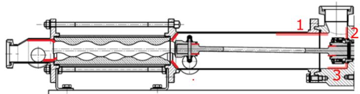
Fig. 1: Critical areas (red) for cleaning in a progressive cavity pump. Presented CFD results for wall zones 1,2 and 3
