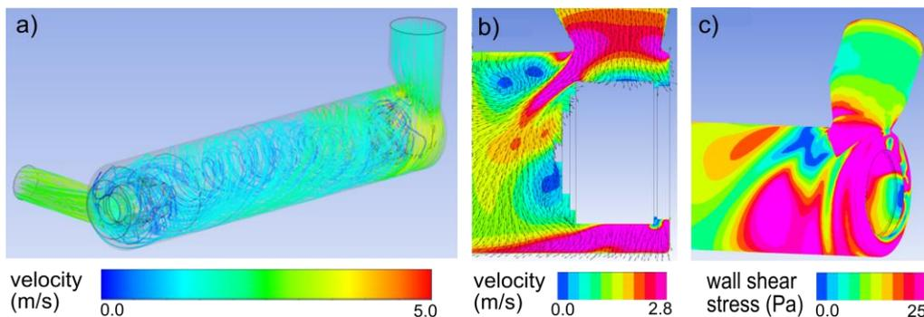
Fig. 2: CFD results for the optimized geometry (case B): a) Streamline plot colored by local velocity; b) velocity contour plots in a cross section at the inlet port area; c) Wall shear stress in a contour plot at outer walls.
