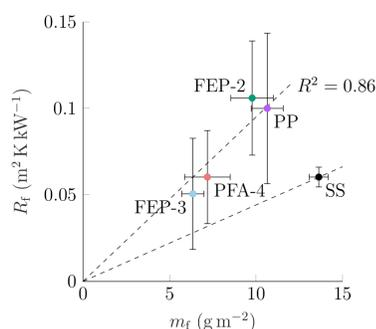
Figure 5: Final fouling resistance over whey protein deposit mass coverage for different surfaces tested with the bench-scale HEX. Dashed lines show root mean square fitted equation  $R_f = m_f / \rho_f k_f$  to find values of  $\rho_f k_f$  for polymer surfaces and stainless steel. For polymer surfaces  $\rho_f k_f = 105\ kg^2\ m^{-2}\ s^{-3}\ K^{-1}$  and for stainless steel  $\rho_f k_f = 226\ kg^2\ m^{-2}\ s^{-3}\ K^{-1}$ . Error bars show 90 % confidence intervals.
