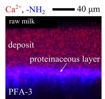
Figure 4: Orthogonal CLSM section of a raw milk fouling layer generated on a perfluoroalkoxy coating.
