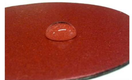
Figure 2: Example of a fluoropolymer antifouling coating in contact with a water droplet.
