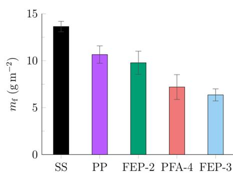
Figure 3: Deposit coverage (dry mass per area) from whey protein solution for different surfaces tested in the bench-scale HEX for a duration of 150 min at a surface temperature of 89 °C. SS – stainless steel, PP – polypropylene, FEP – fluorinated ethylene propylene, PFA – perfluoroalkoxy. Error bars show 90 % confidence intervals.
