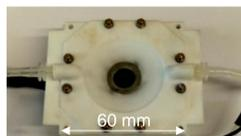
Screening experiments with **micro scale heat exchanger**
