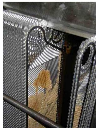
Figure 1: Milk fouling in a plate heat exchanger.
